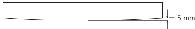
Figure 4.23: Sketch of the observed bulging shape of the old rubber tool at 65^\circ\text{C}
